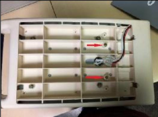
You will now see a couple of screws when you remove the lid on the top side of the hood. Unscrew the 2 screws as shown on the picture with a Philips screw driver while holding the knife assembly from the other side. Use protective gloves to hold the knife assembly.
